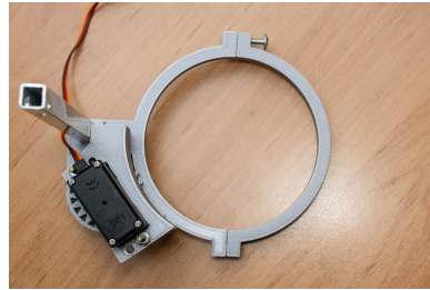
(b) : mStructF-arm for holding the DRC (without DRC on picture)
