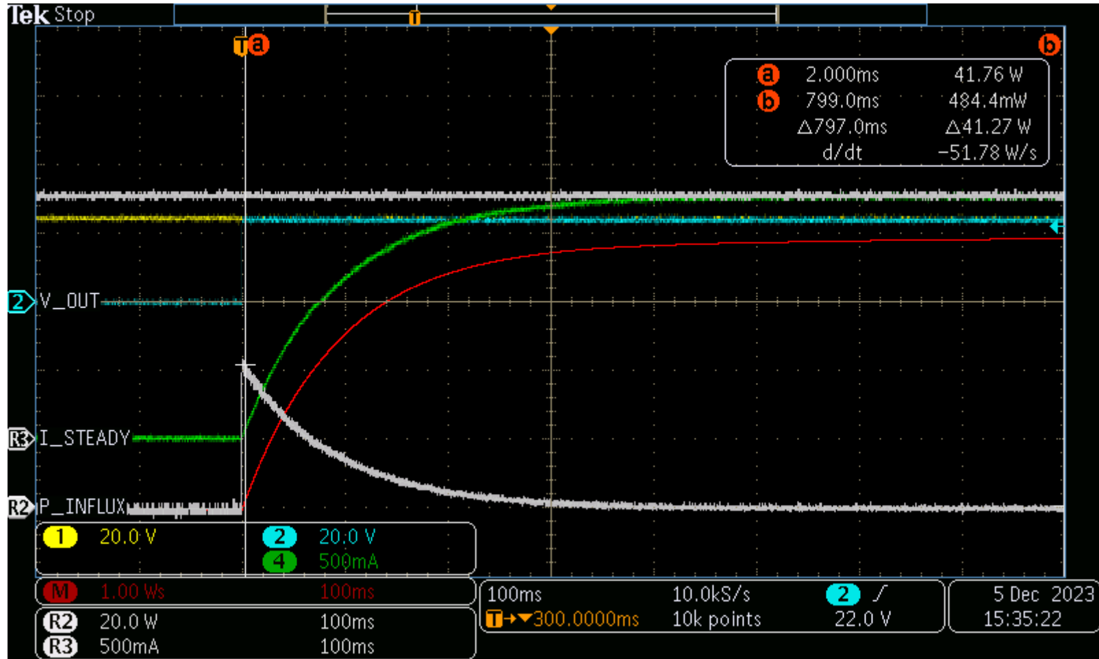
FIGURE C.3: SWITCHING ON A 1.2H(14 \Omega ) INDUCTOR
