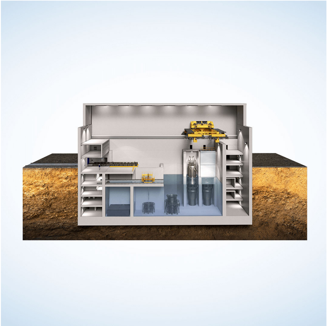
Fig. 2.2: VOYGR-4 reactor hall scheme [11]
