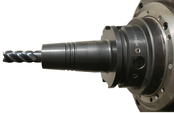
Figure 9.4: ISCAR EC120B25-4C12 IC900 flat-end mill in SCHUNK TENDO Slim 4ax HSK-A63 \text{\O}12 \times 120 hydraulic tool holder
