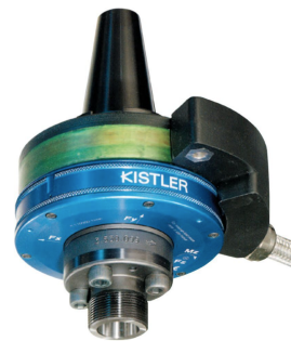
(b) Rotary dynamometer Kistler 9123C [55]
