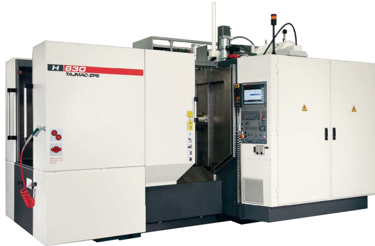
Figure 9.1: TAJMAC-ZPS H630 horizontal machining centre [79]
