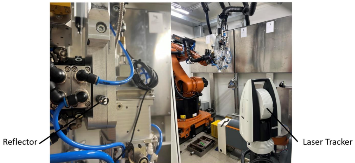
Figure 8-6: Laser tracker setup
