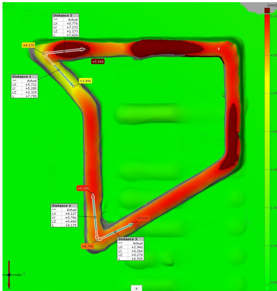
Figure 9-8: Material accumulation due to wire speed acceleration and movement interruption
