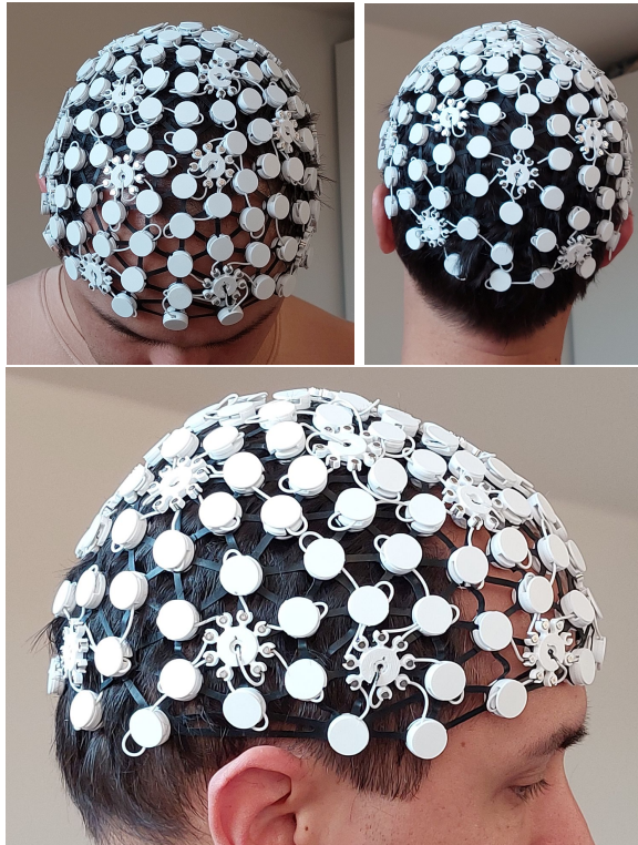
Figure 7.3: The cap with electrodes without electronics Pictures provided by the thesis supervisor
