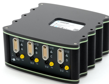
Figure 2.7: An amplifier unit from g.tec[g.tmp]
