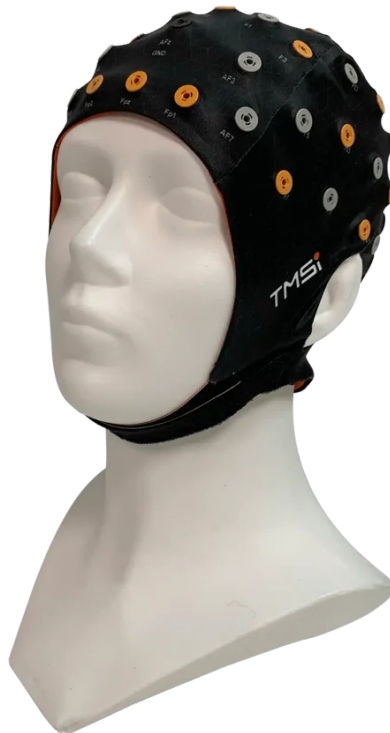
Figure 2.3: Example of gel electrodes in a cap[Elees]
