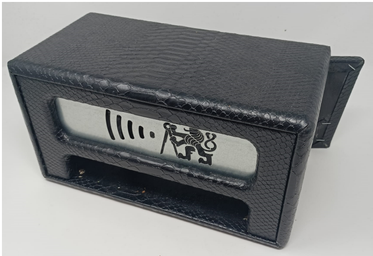
Figure 7.1: Photo of the wooden tolex-coated shell.
