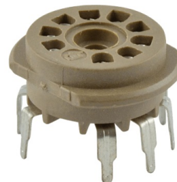
(f) : Tube socket Noval Belton, Print VT9.[33]
