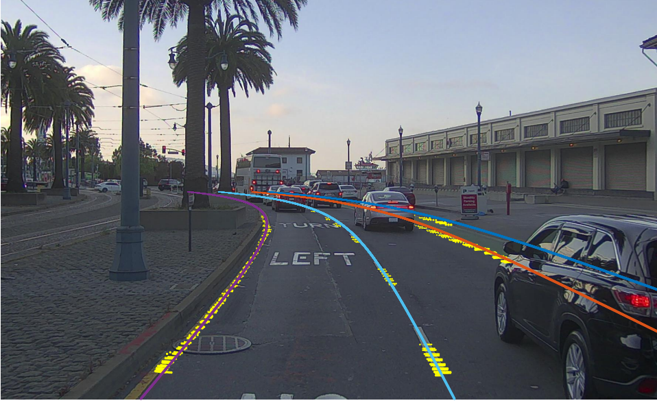
Figure 3.20: Projection of the estimated lines and LIDAR detections (yellow dots) onto the image.
