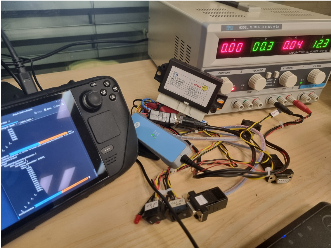
Figure 1.2. Photo of Bosch PDU Parking ECU, on which most of the tests were carried out
