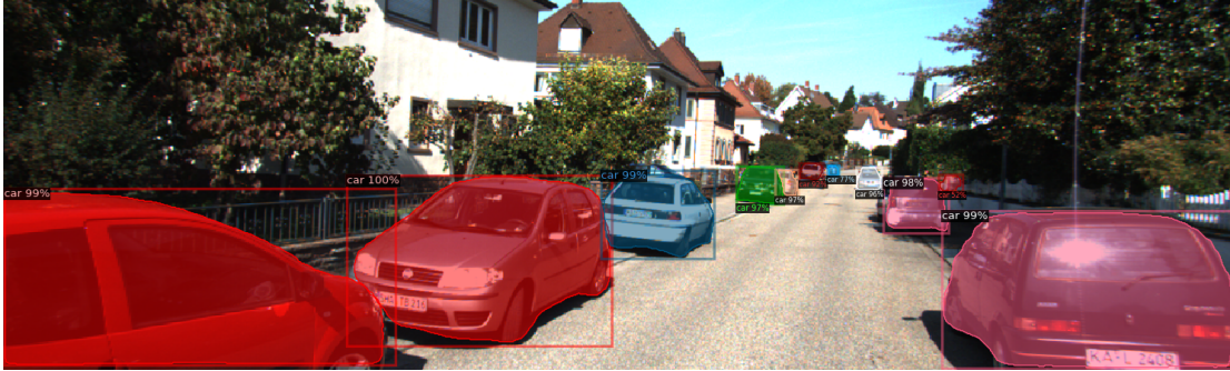
Figure 3.1. Example of using Detectron2 [35] framework as instance segmentation tool on KITTI [3] dataset.
