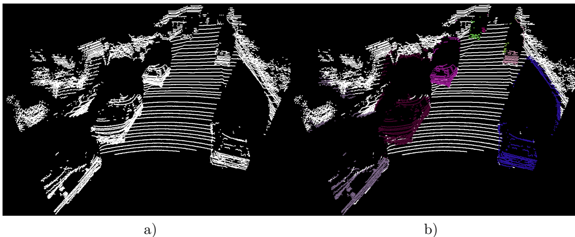
Figure 3.4. Example of the foreground segmentation. (a) raw point cloud (LiDAR scan) cropped to camera FOV, (b) foreground segmentation performed on all objects visible in the camera. Each distinct color represents a different object instance.
