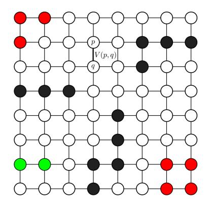
**Figure 4.2:** The graph in this figure is represents the situation in Figure 4.1b. Each node corresponds to a pixel and edges are only present between neighboring pixels. The weight between two neighboring pixels, p and q, denoted as V(p,q) and is set according to the equation 4.1, which depends on the intensity of the pixels.
