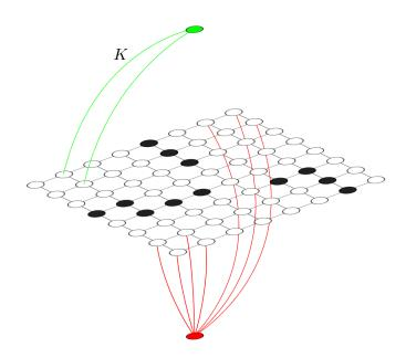
Figure 4.3: The figure illustrates how the assignment of the sink and source pixels are assigned to graph in Figure 4.2. The data term K is assigned to the edges between the source/sink and the scribbled pixels, while the edges between the source/sink and the other pixels have set a value of 0, indicating no connection to the source/sink.
