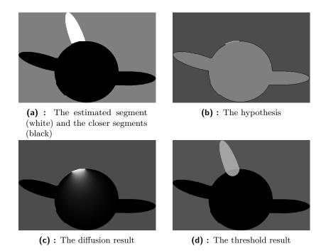
**Figure 3.9:** The task we aim to solve is to recreate shape of the overlapped segment marked by the white area in picture (**a**). Picture (**b**) displays the boundary conditions that will be diffused. The white and black pixels represent the boundary conditions and the light-gray area is used for computation. The diffusion result for the blue segment can be found in image (**c**), while the thresholded diffusion results for the overlapped segment are displayed in picture (**d**).
