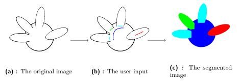
**Figure 3.1:** In the figure we can see the segmentation process. The user adds scribbles to the image, as can be seen in image (b). The segmentation process then fills the contours with the color of the drawn scribbles.
