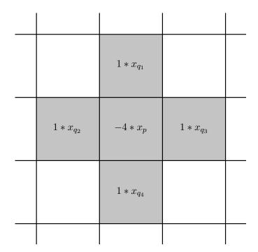
**Figure 3.10:** The Laplacian of the image is calculated using the 4-neighborhood of the pixels. The sum of the coefficients in all pixels of the 4-neighborhood, including the pixel  $x_p$  and its neighboring pixels  $x_{q_i}$  where  $i \in \{1, 2, 3, 4\}$ , is equal to zero.
