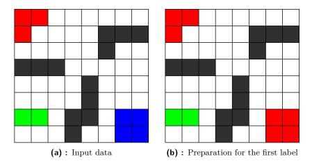
**Figure 4.1:** The figure shows the initialization of the LazyBrush algorithm. The user input is contained in the 8x8 grayscale image (a). The input consists of three labels: blue, red and green. The dark pixels in the image represent contours. Figure (b) is used to prepare the input for the computation of the green segment.
