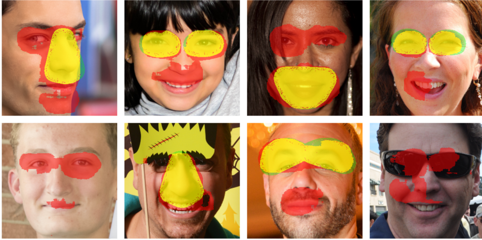
Figure 4.15: Results of localization of fake areas in the images with U-Net model. The red areas are incorrect predictions of the fake areas (false positives), green areas are ground truth fake areas undetected by our model (false negatives), and yellow areas are where our model correctly localized the fake areas (true positives).
