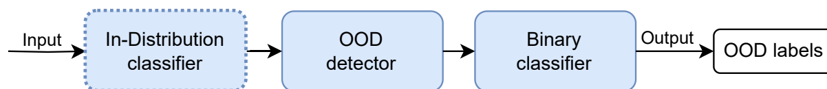
Figure 4.1: High-level OOD detection overview. An OOD detector takes the Compounds or Test datasets, optionally processed by a ID classifier, to produce OOD scores. A binary classifier then takes the scores as input and returns OOD labels. The labels denote whether an input is In-Distribution or Out-Of-Distribution.
