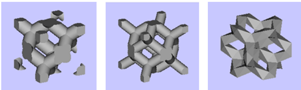
Figure 28: Geometry of BECs of individual specimens: left—Diamond, center—Rhombic, right—Dode Thick. Figure taken from a co-authored published work [124].
