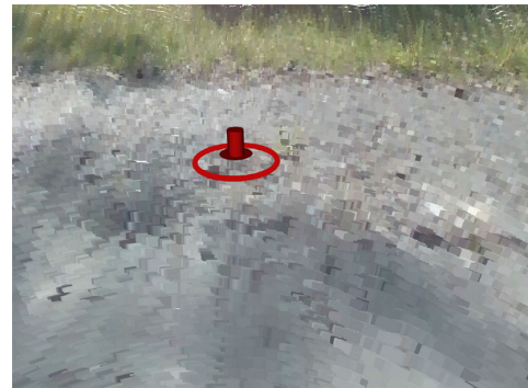
Fig. 15 The area (red circle) around a point of interest (red marker) signifying the cells used to compute the histogram terrain descriptor, projected on the elevation map with localized color measurements (Color figure online)
