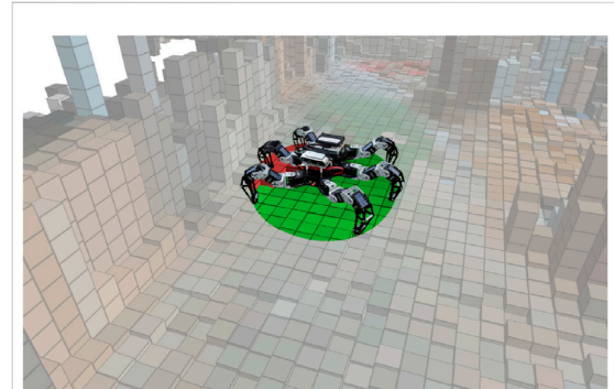
FIGURE 2 Footprint around the robot position covers the cells with potential multi-legged walking robot footholds.
