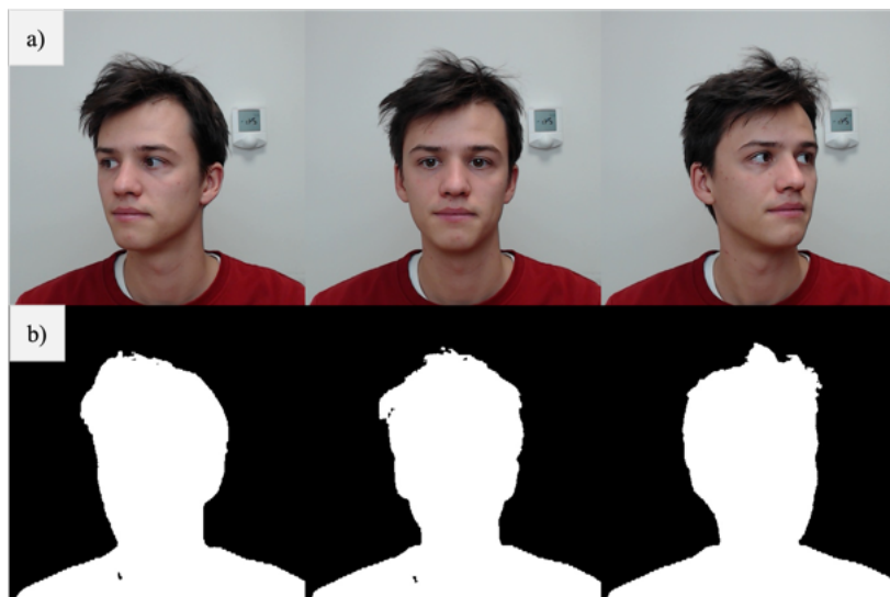
Figure 4.6: Foreground masks created using the MediaPipe selfie segmenter. a) contains the input keyframes from which the training masks b) are created.
