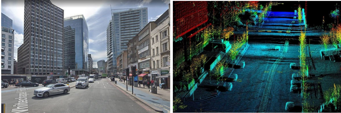
(a) An image from the Google Street View website [12] (b) A point cloud map generated from LiDAR sensor data [13]
