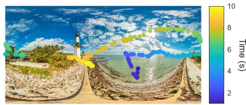
Figure 7.8: Observing an individual's gaze synchronized with a relevant background image. The figure also depicts gaze position based on time by utilizing time data.
