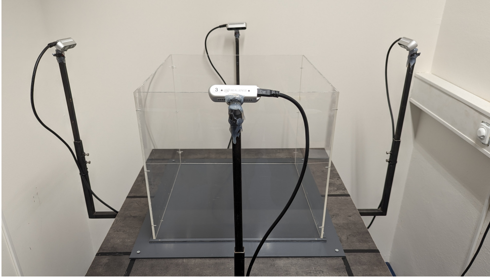
Figure 2.1. The setup of the quad view camera system built for capturing our experiment video footage.
