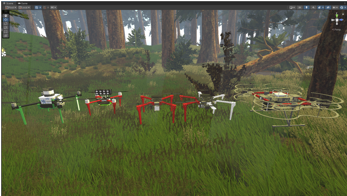
Figure 2.10: Drone models available in the framework, from left to right: X500 , F330 , F450 , F550 and NAKI II
