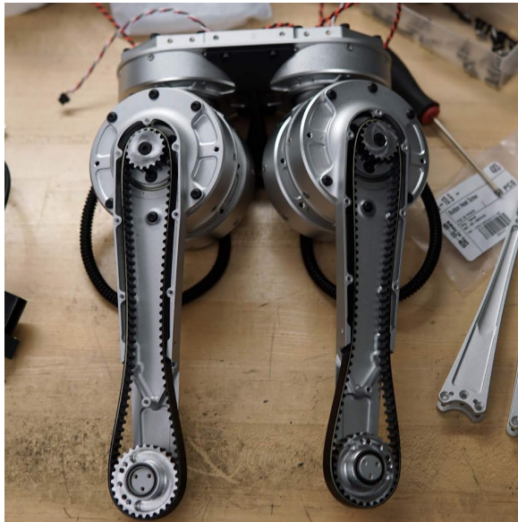
(b) : Assembly of the Cheetah robot's legs, showcasing the belt drive actuation [19]
