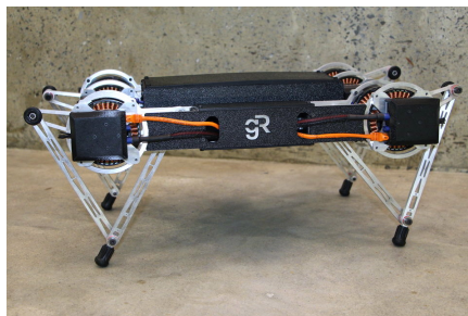
(b) : The robot Minitaur as constructed by Ghost Robotics [23]
