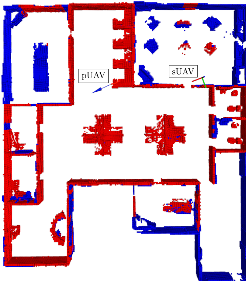
Figure 4.2: Occupancy map of the office space at the end of the 4-minute mission. The red color represents an area scanned by the pUAV using LiDAR, the blue color represents space explored only by sUAV.
