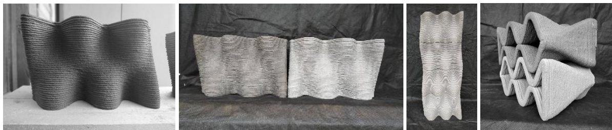
Fig.62. a) High-quality layers of panel MinSurf using L5W18 layer b) Widening gap between two panels, caused by inclined walls c) Set of four panels d) Second option of panel assembly
