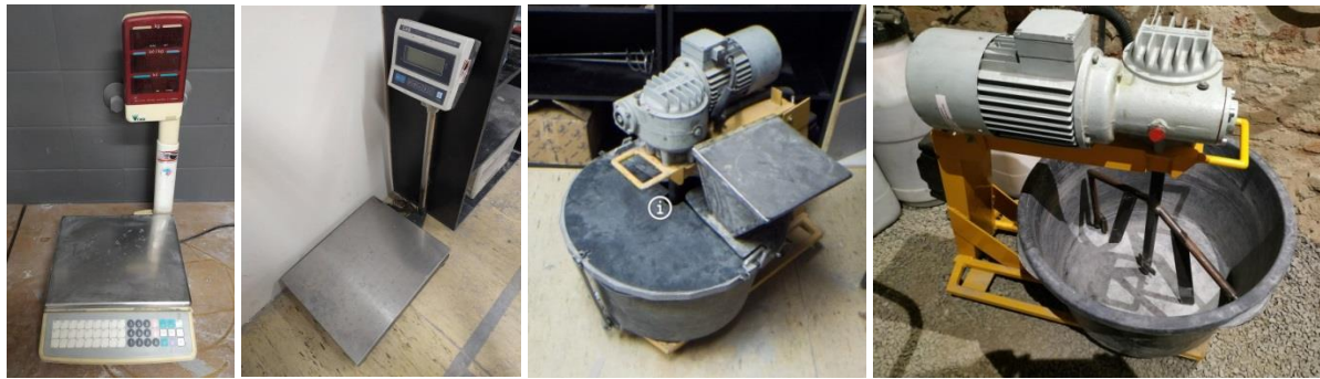
Fig.31. a) DS608 scale b) CAS DB2 bridge scale c) Bespoke mixing station- Fresh mixing setup d) Dry mixing setup
