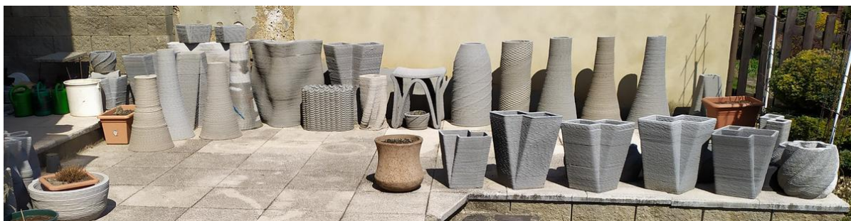
Fig.100. Illustrative selection of printouts from various materials, fabricated during 3 years of a 3DCP research as a part of this thesis
