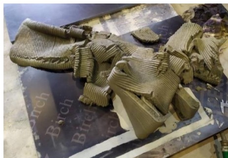
Fig.83. Collapse of the H-O vase No.3 during printing due to depletion of shear strength
