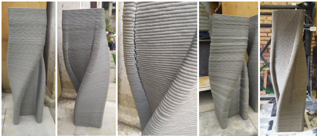
Fig.82. H-O vase printouts a) No.1 - side without cracks b) No.1 - Side with shear crack. c) No.2 – Layer profiling due to mixing of small batches d) No.4 - High-quality print of adjusted model e) Hardened H-O vase No.1 – Detail of cracks
