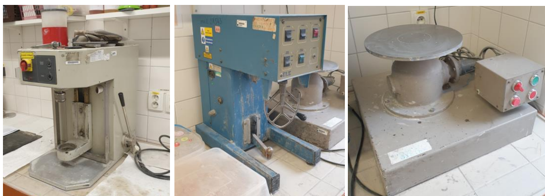
Fig.24. Small scale testing equipment a), b) Standard lab mixers c) Flow test apparatus
