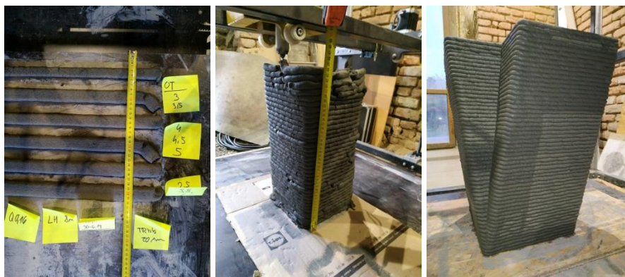
Fig.50. a) v - f script test with CM276 b) Improving buildability and quality by adjustments of recipe
