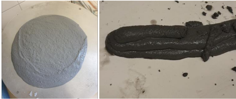
Fig.89. Results of small-scale testing of SF350c a) Flow b) Extrusion test
