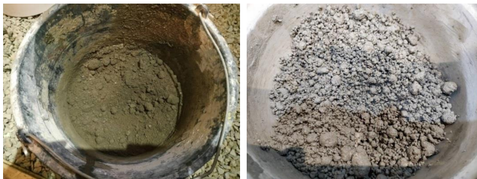
Fig.47. a) Consequence of inappropriate mixing procedure - adding water with plasticizer to the whole batch of dry mixture leads to the formation of dry mixture with lumps. b) Temporary change in consistency after addition of VMA - formation of spherical lumps
