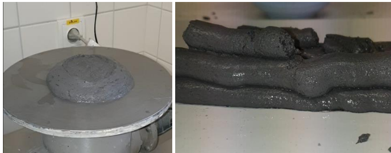
Fig.95. Results of small-scale testing of SF550c a) Flow b) Extrusion test
