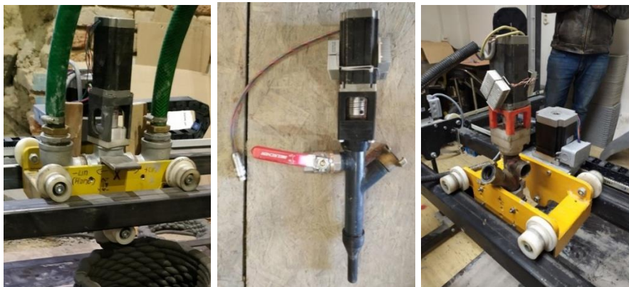
Fig.41. a) PH3 with material discharge without pressure control b) PH4 with infinitely adjustable material discharge for nozzle pressure control c) PH5 with discharge perpendicular to the side
