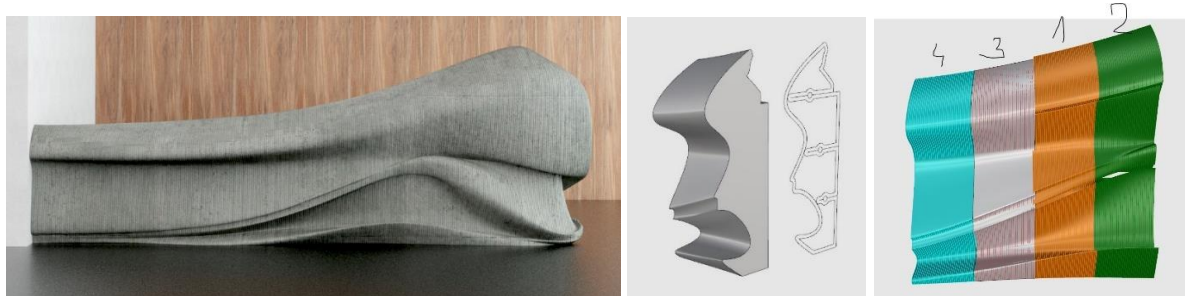
Fig.57. a) Visualisation of the reception desk (by Dominik Císař) b) Model section and layer incl. reinforcements c) Reception desk panelization showing division into four panels
