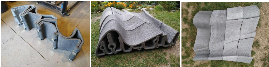
Fig.60. a) Panel 2 assembled of smaller parts 2A, 2B, 2C b) c) Set of printed panels 1(A+B+C)+2(A+B+C)+3+4 , displaying various quality
