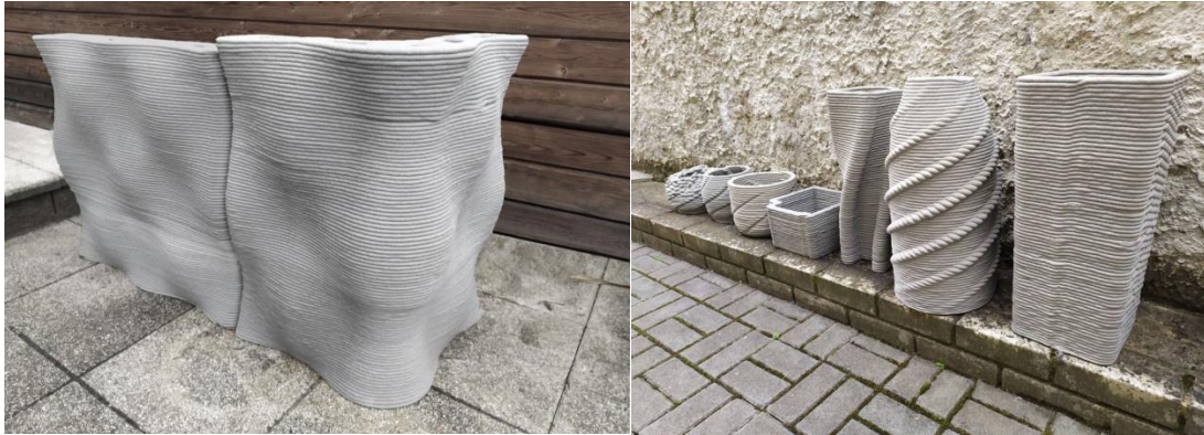
Fig.84. a) PAN_SIN, corner element (180kg) b) Various vases with L8/W18-22 in high-quality
