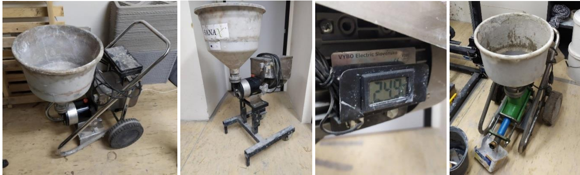
Fig.32. a) Pump S8 b) Upgraded pump S8 c) Thermometer on S8 motor d) Pump DT
