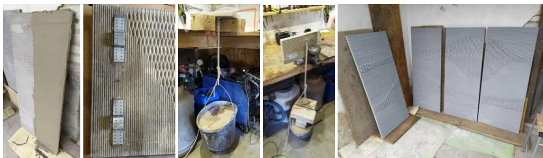
Fig.73. a) Panel reverse side with reinforcing mesh and 2mm squeegee b) Anchor profiles glued to the reverse of the panel c) Indicative test of the pull-off force perpendicular to the panel d) Indicative test of the pull-off force along the panel e) Set of finished panels coated with MasterProtect H 321 prior to the final delivery
