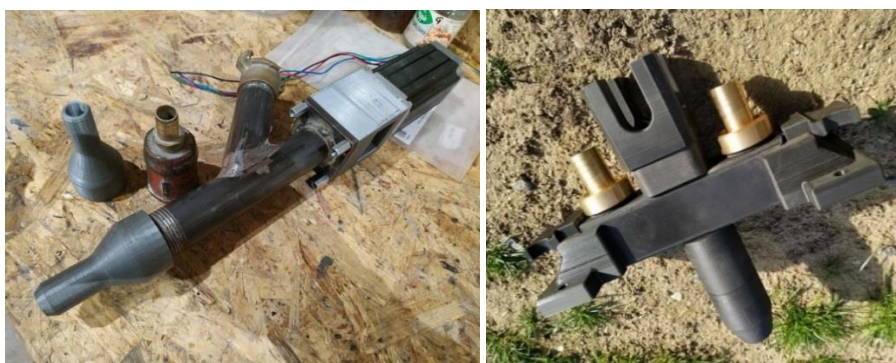
Fig.40. a) PH1 with interchangeable nozzles b) PH 2 with pressure control by material discharge
