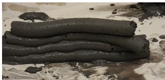
Fig.88. Results of small-scale testing of SF350b a) Extrusion test
