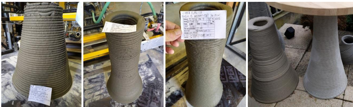
Fig.76. a) On the left, layer variation of a print of TAM model from Flow 3D 100, on the right the same model from Flow 3D 100 with HCA, treated with Kure 220WB - uniform layers, but spots b) Print log of TAM script using 2x18kg batch c) 1x36kg batch of Flow 3D 100
