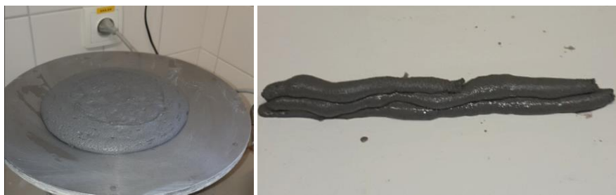
Fig.92. Results of small-scale testing of SF450c a) Flow b) Extrusion test
