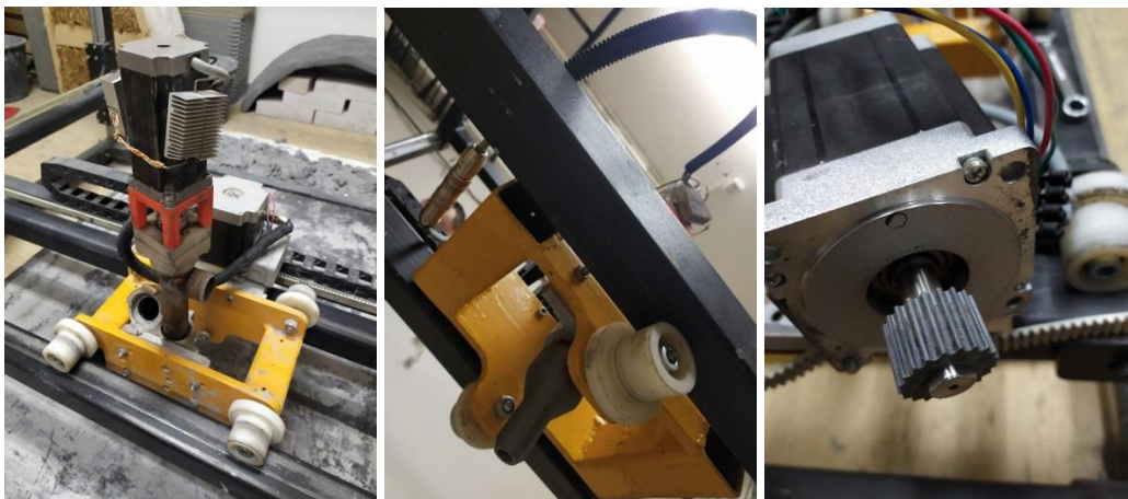
Fig.38. a) X axis cart, carrying PH5 b) X axis cart from below, with nozzle TP11 c) Detail of 3D printed shepherd on X axis motor
