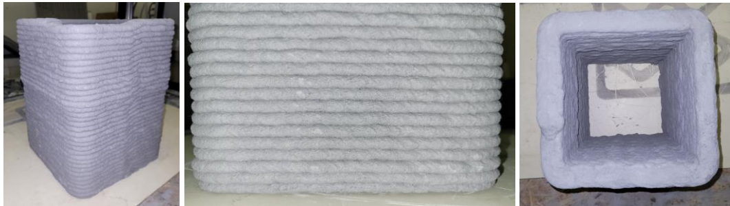
Fig.97. Mixture SF450c a) View of the individual layers of the specimen b) Detail of the layers at the bottom of the specimen c) Detail of the shape of the layers of the print specimen from above
