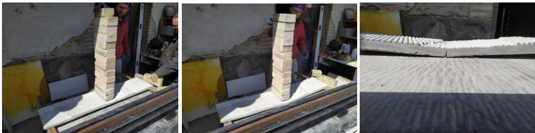
Fig.72. a) Indicative flexural tensile strength test a) Loading of reinforced panel b) Maximum load of reinforced panel at failure c) Detail of failure of reinforced panel
