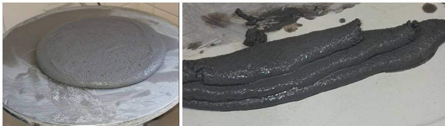
Fig.90. Results of small-scale testing of SF450a a) Flow b) Extrusion test
