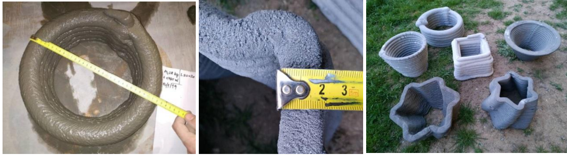
Fig.51. Printing with mixture CM276 by its extrusion from a pipe a) First print – thick layer b) Thin layers after 1 month of development c) Print examples
