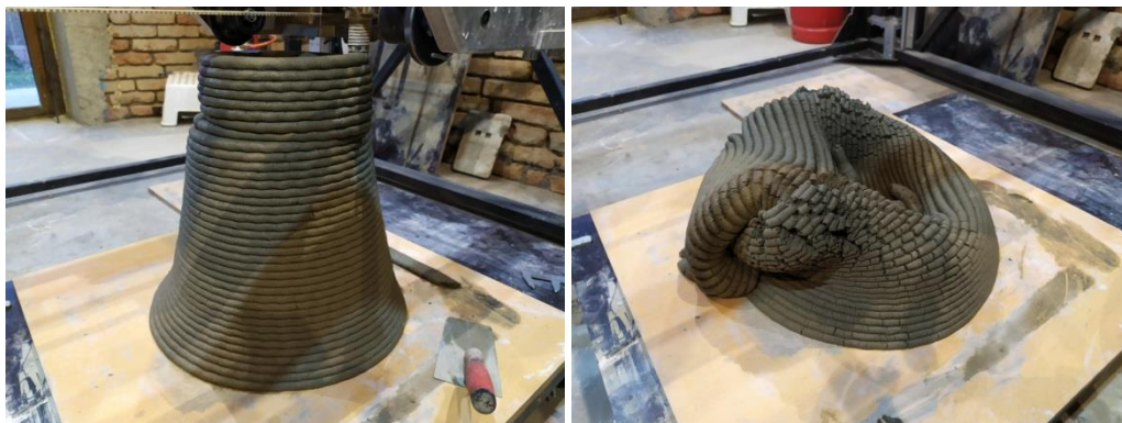
Fig.30. Collapse of TAM geometry during printing process due to an error of printer, causing unexpected layer eccentricities on top
