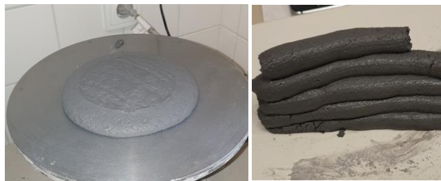
Fig.91. Results of small-scale testing of SF450b a) Flow b) Extrusion test
