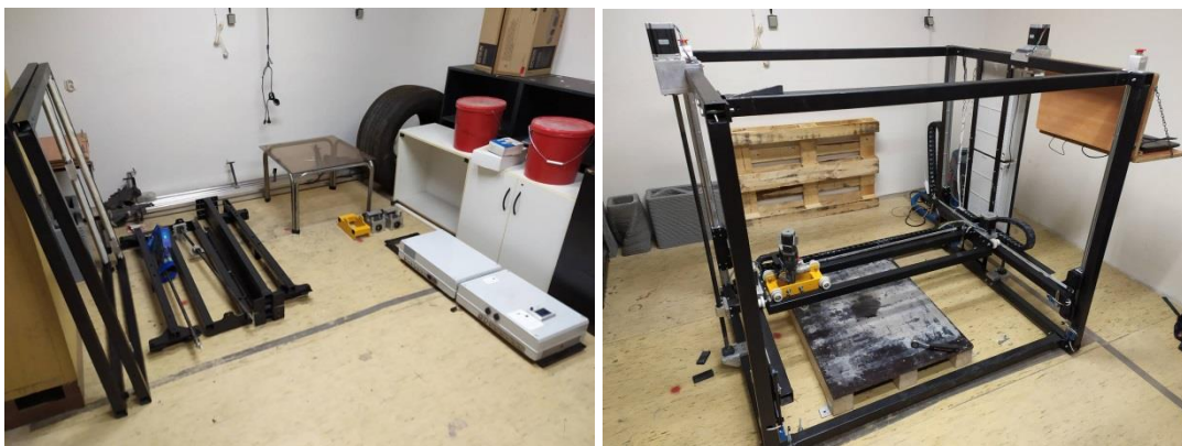
Fig.34. a) 3D printer parts before assembly b) Assembled 3D printer, carrying PH5
