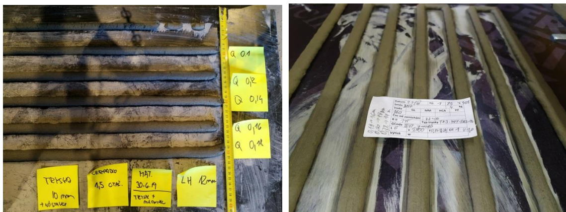
Fig.29. a) Test print to find the optimum extrusion coefficient f with the resulting miniprotocol b) Testing trajectories for testing of v/f parameters according to v-f script
