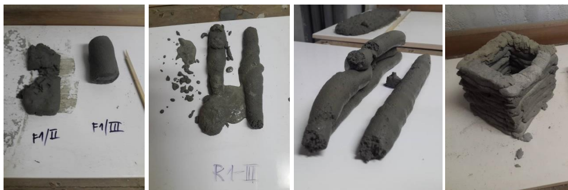
Fig.44. The result of Redrock mixture extrusion test by sealant gun Powerfix Profi a) Batches F1/II and F1/III b) R1-III c) d) P1-II
