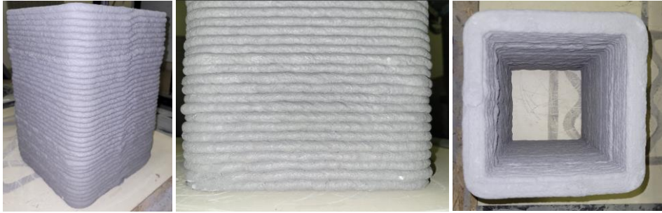
Fig.96. Mixture SF450b a) View of the individual layers of the specimen b) Detail of the layers at the bottom of the specimen c) Detail of the shape of the layers of the print specimen from above
