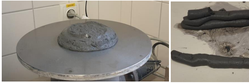
Fig.94. Results of small-scale testing of SF550b a) Flow b) Extrusion test
