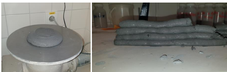
Fig.93. Results of small-scale testing of SF550a a) Flow b) Extrusion test
