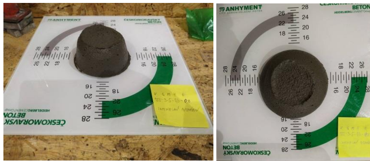
Fig.48. Simplified flow test of CM276-123-3-5-0.6-0.8 (modified by admixtures:123 g W, 3g MG, 5gMM, 0.6gHCA, 0.8g MF6). Flow value 150 mm.
