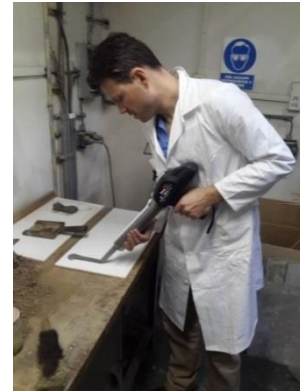
Fig.26. a) The extrudability/buildability testing procedure in a small scale using the sealant gun b) The author using pistol Skillmaster for testing of extrudability of mortar
