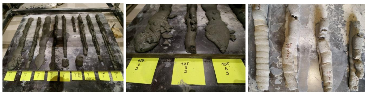
Fig.45.a) b) c) The results of extrusion tests using sealant gun Powerfix Profi
