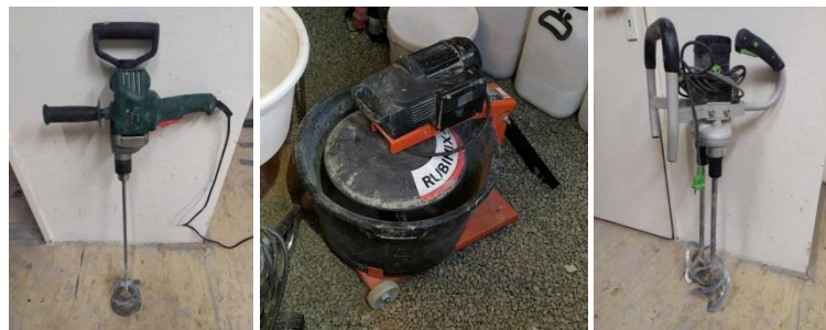
Fig.15. a) DWT BM-720 M gear stirrer with a mixing whisk b) RUBI Rubimix 50 N mixing station c) Gear stirrer FESTOOL MX 1600/2 EQ DUO
