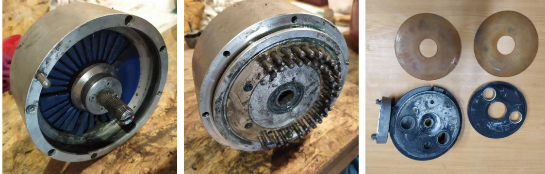
Fig.33. a) Peristaltic lamellas of S8 pump b) Pins of S8 pump, worn out after 400 machine-hours. c) Internal worn-out front cover and sealing rings.
