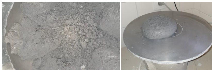
Fig.87. Results of small-scale testing of SF350a a) Consistence at the end of mixing b) Flow
