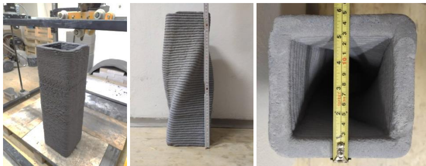
Fig.99. a) Test of buildability – printing of SF550c up to the height 750mm b) c) High quality print of H-O_050 vase with the height 440mm – SF450b
