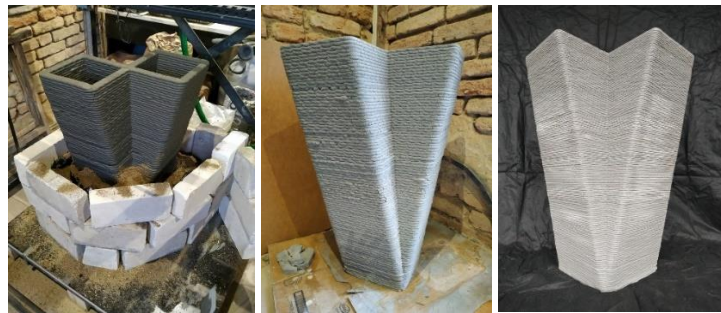
Fig.56. a) Printout of V vase L8/W25 with layers supported during printing by sand backfill b) Hardened printout after 2 weeks c) Hardened V vase L5/W25
