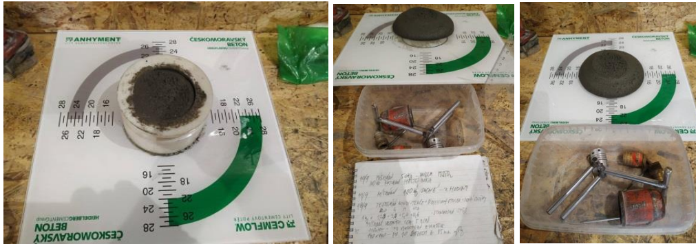
Fig.28. Simplified test apparatus and demonstration of the flow test for an indicative check of the consistency of the mixture before printing
