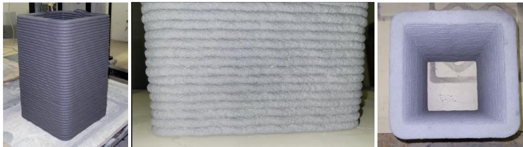
Fig.98. Mixture SF550c a) View of the individual layers of the specimen b) Detail of the layers at the bottom of the specimen c) Detail of the layers of the print specimen from above
