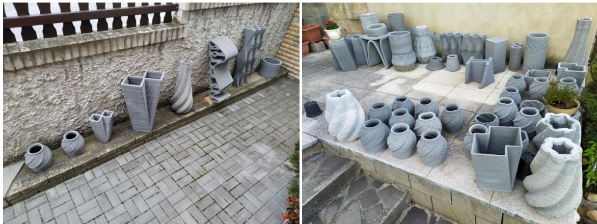
Fig.64. Examples of prints from CM276 mixture a) High-quality prints b) Illustrative set of prints
