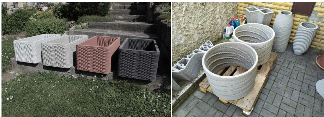
Fig.85. a) Set of coloured planters with L8/W18 b) Big planters with L8/W25, d=600mm, batch 60kg, four prints in four tasks, uniform appearance, high-quality
