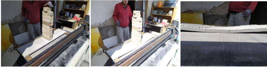
Fig.71. a) Indicative flexural tensile strength test a) Loading of unreinforced panel b) Maximum load of unreinforced panel at failure c) Detail of failure of unreinforced panel
