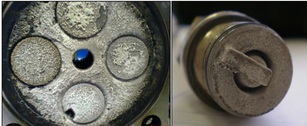
Figure 14. Siloxane influence on engines [52].
