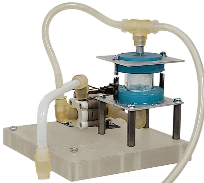
Figure 2.6: Particle injector for flow visualisation.
