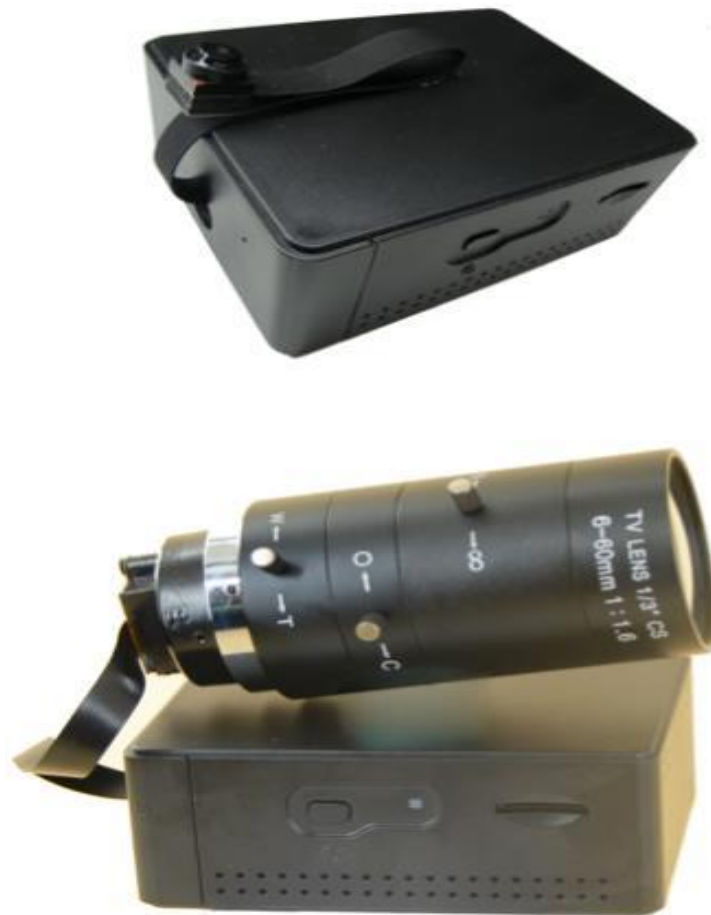
Figure 4.9 The WIFI camera before and after replacing the lens [23].
