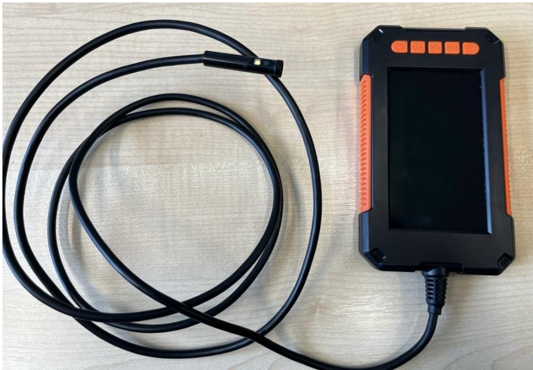
Figure 4.16 Screen of the dual-lens endoscope [photo – author].
