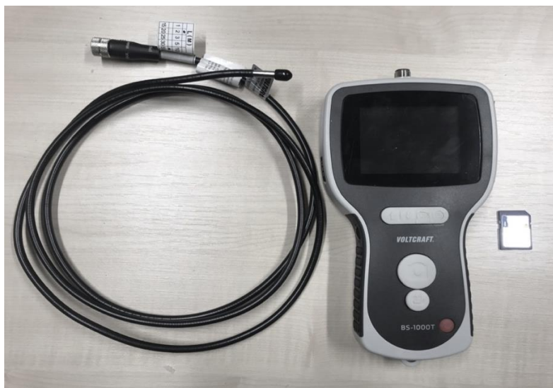
Figure 4.10 Semi-rigid endoscope with the monitor and the memory card [photo – author] .
