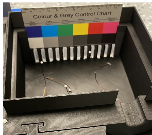
Figure 5: Detail of cavity with polyp holders and colour chart
