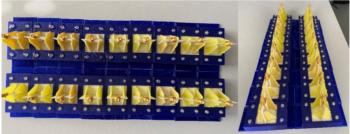
Figure 4.11: UWB antenna components with a 3-D printed holder attached.
