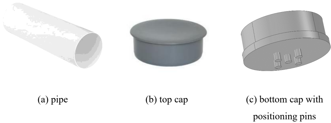
Figure 4.9: Components used for the container holding the increased temperature phantom [33].
