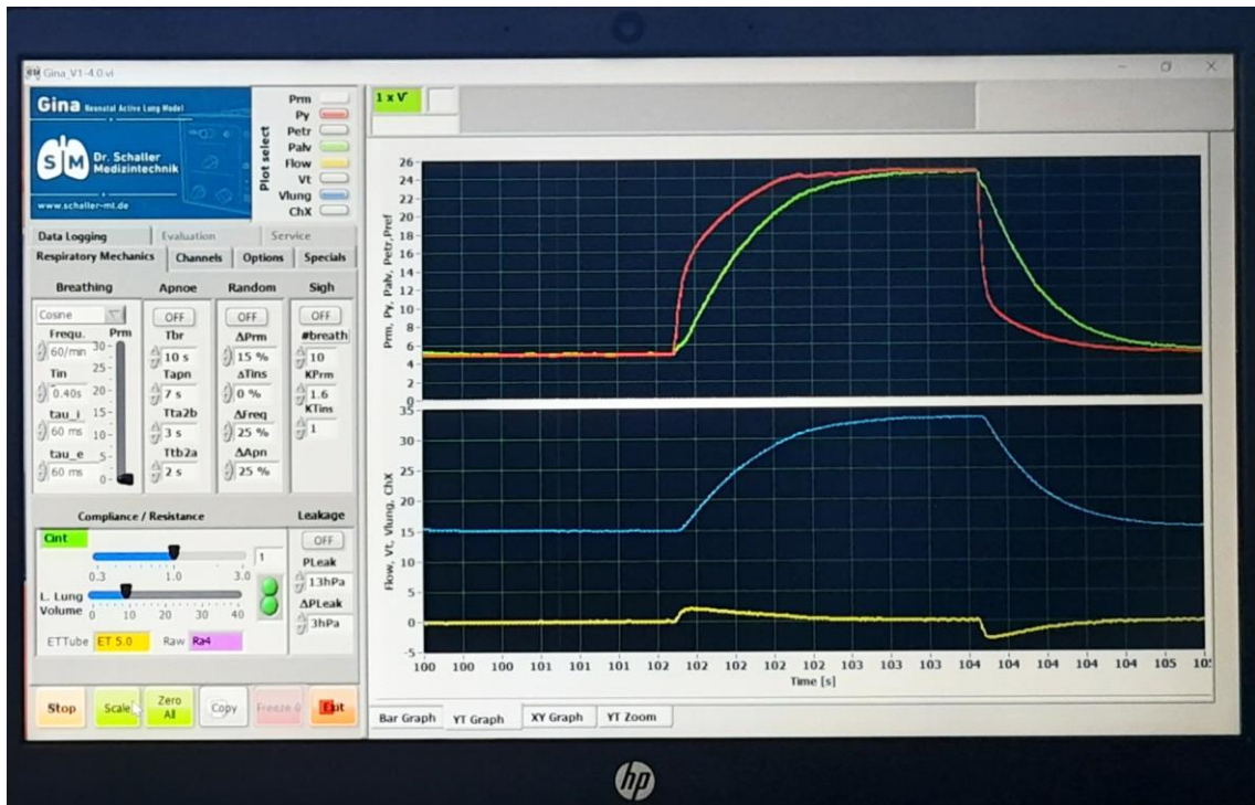
Figure 4.9: GINA simulator interface shows the chosen compliance value with a clear graphical representation of the applied pressures (green line in the upper window - P_y ; red line in the upper window - P_{alv} ). Photograph: author.
