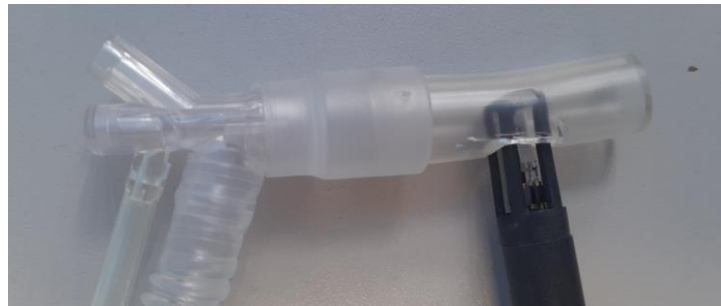
Figure 4.13: Insertion of TESTO 635 into rPAP T-piece. Photograph: author.
