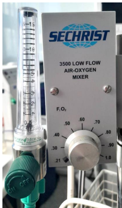
Figure 4.5: Mixer Sechrist 3500 and flowmeter Oxygen Chrome used in the practical experiment. Photograph: author.
