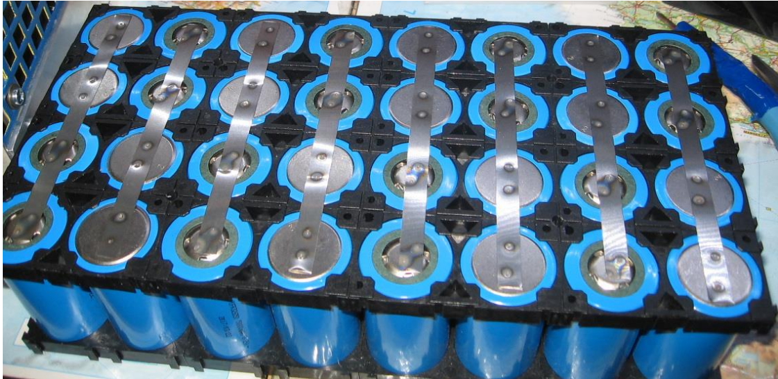
Fig. 5 Example of 500 Wh battery pack of lithium cells
