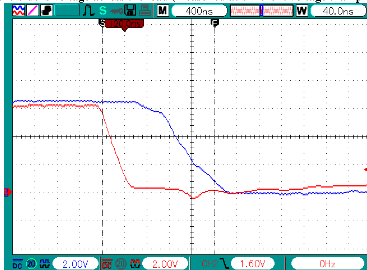
Fig. 36 Slow gate discharge after over-current detected. The blue is voltage at the gate and red comparator output to show when the over-current was detected
