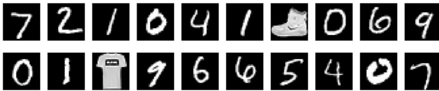
Figure 1.5: Images from MNIST as the normal data and 2 images from Fashion-MNIST as the anomaly data. [22]
