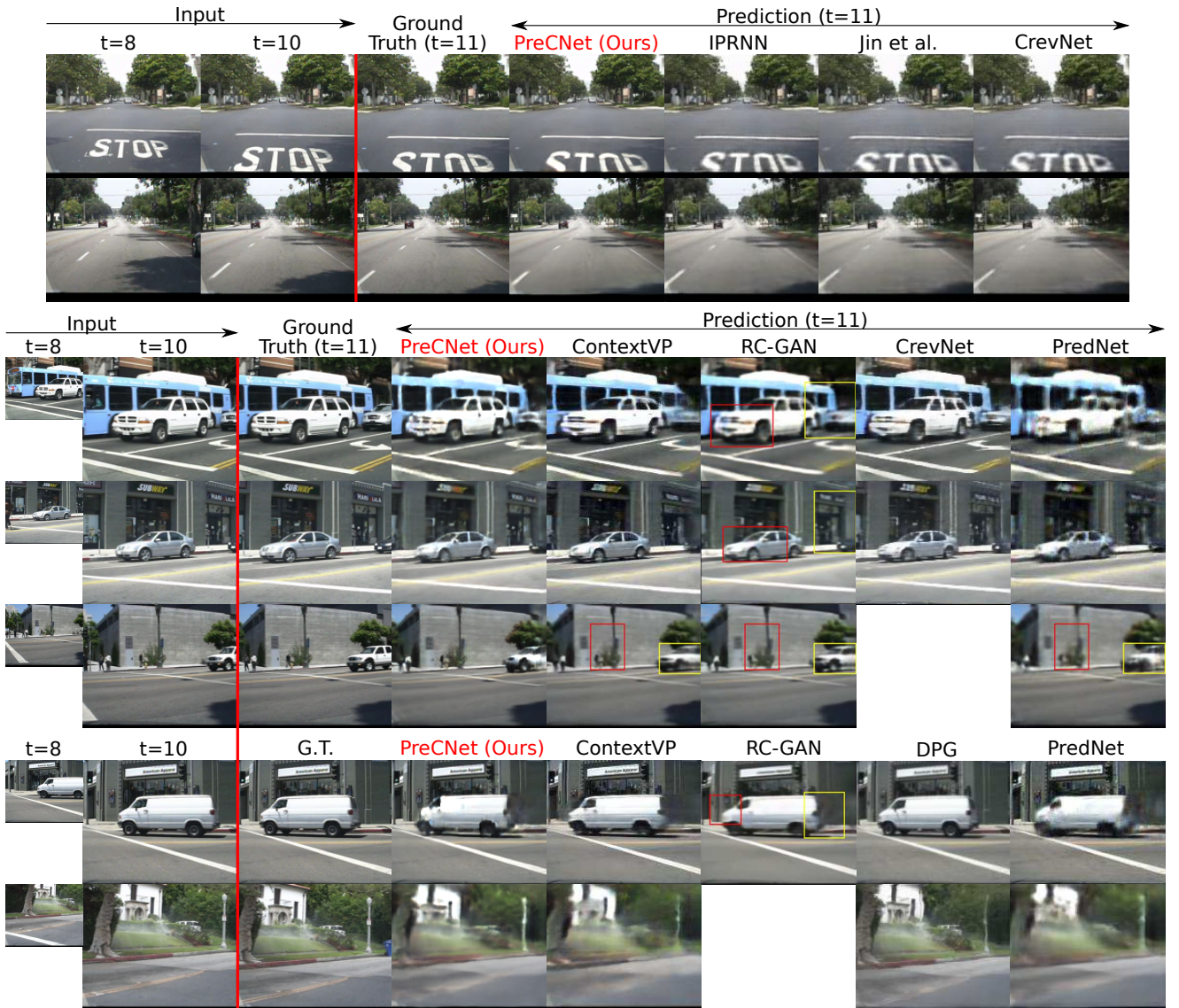
Fig. 5. Qualitative comparison of PreCNet with others state-of-the-art methods on Caltech Pedestrian Dataset. All models were trained on KITTI dataset. Ten input frames were given (see frames for t = 8, t = 10 ), the next one ( t = 11 ) was predicted (RC-GAN used only four input frames – see Section IV-C4 for explanation) by the models (for references see Table III). The images of predictions of other models are copied from original or other cited papers (see references in Table III). Position of the sequences in Caltech Pedestrian Dataset by rows; set06-v013, set06-v000, set07-v011, set10-v010, set10-v009, set10-v010, set06-v009.
