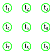
Fig. 5. Schematic illustration of a 3 \times 3 skin patch with 9 taxels.
