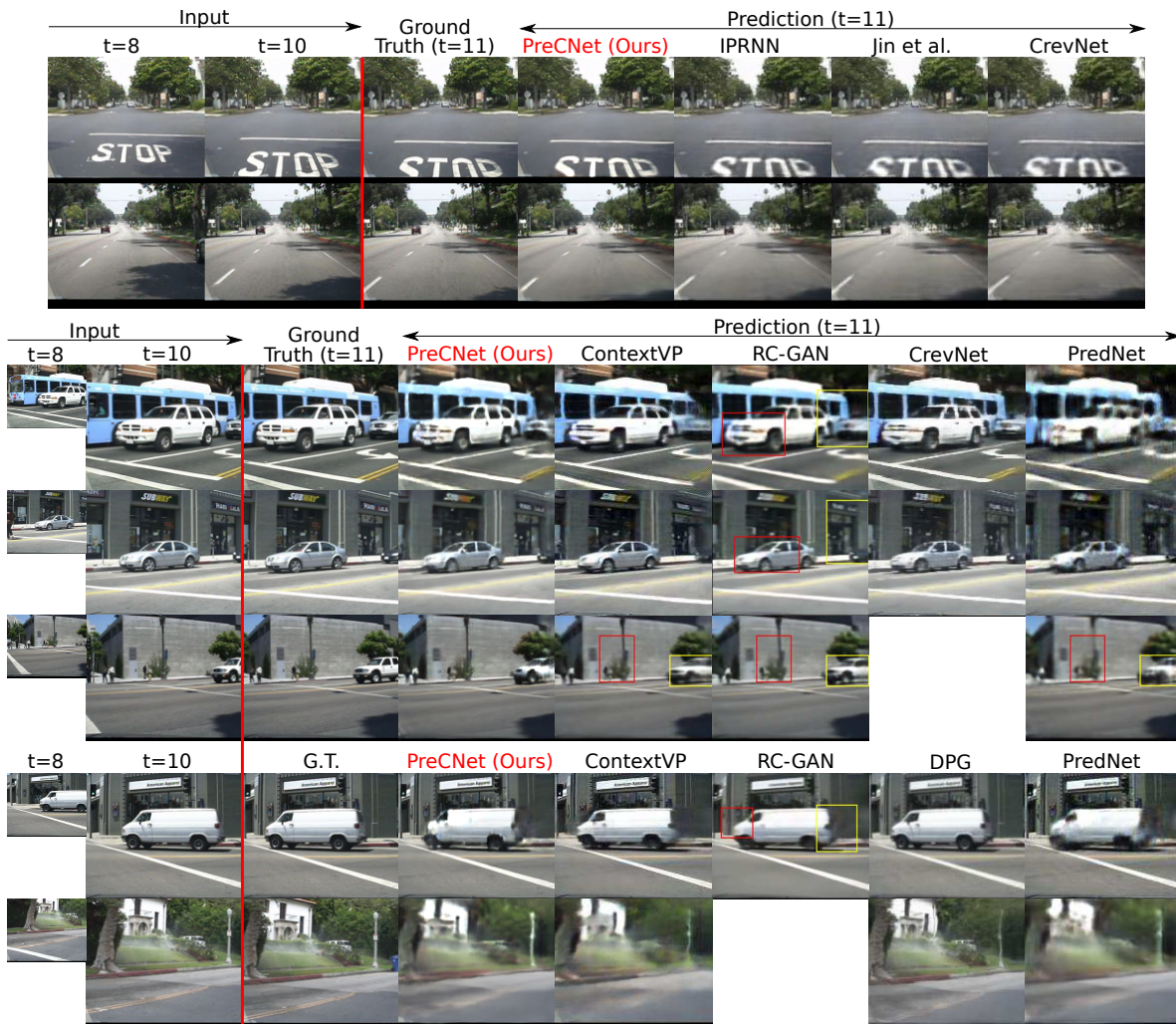
Figure 2.4: Qualitative comparison of PreCNet with other state-of-the-art methods on the Caltech Pedestrian Dataset. Ten input frames were given (see frames for t = 8 , t = 10 ), and the next one ( t = 11 ) was predicted (RC-GAN used only four input frames) by the models (for references, see [36]). Figure and caption (with modifications) from [36].
