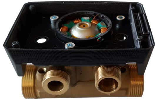
Figure 6.7.: Final brass-casted PCP prototype with the D5 pump stripped of electronics.
