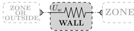
Figure 12.3.: Wall submodel with a thermodynamic circuit. The wall can divide off two adjacent zones or a zone with the outside environment.
