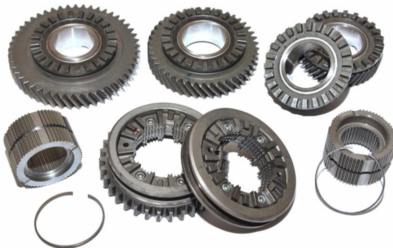
Figure 7: Prototypes of the clutch for the 1st, 2nd, 3rd and 4th gear
