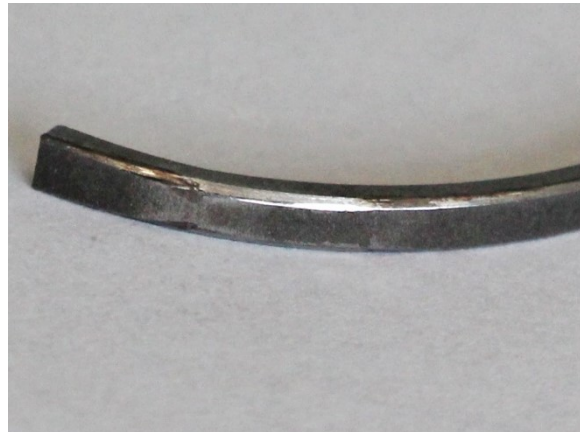
Figure 98: Ring after service life test – detail
