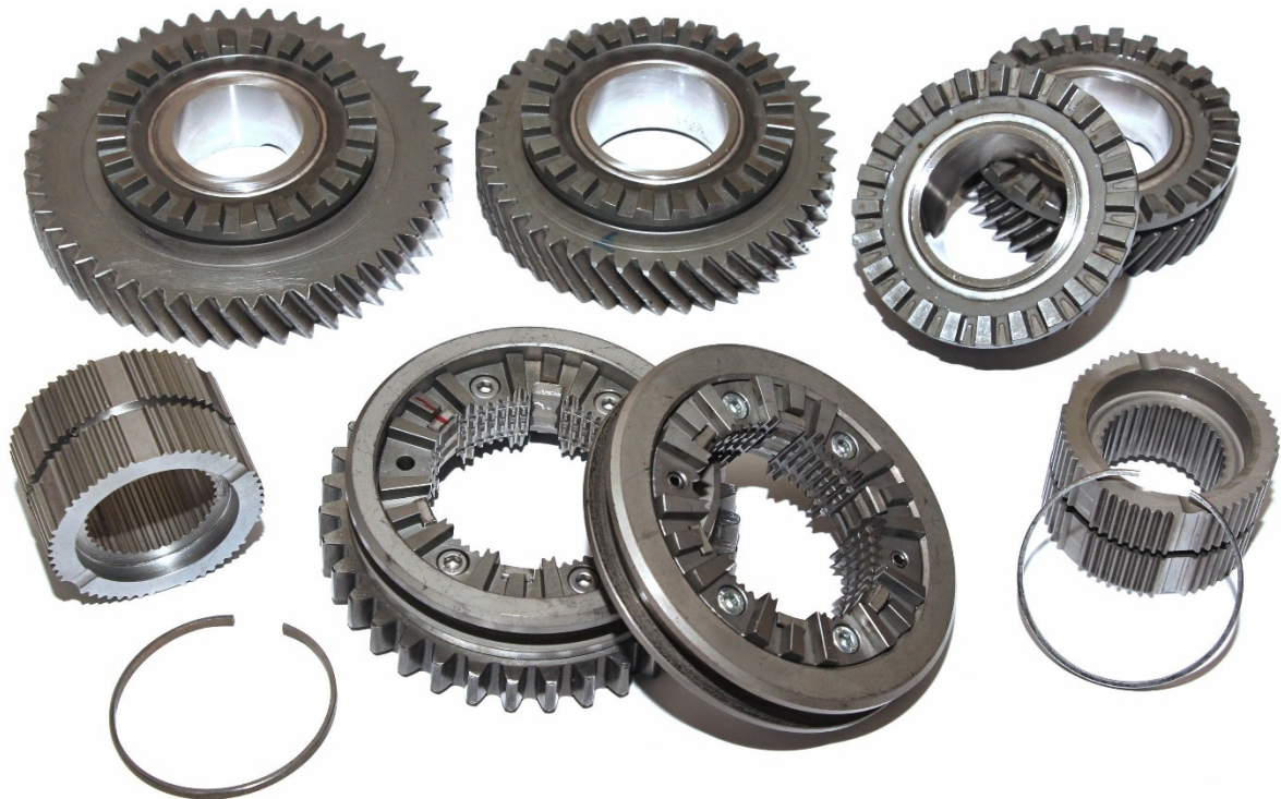
Figure 73: Prototypes of the clutch for the 1 st , 2 nd , 3 rd and 4 th gear
