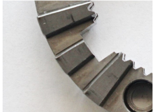
Figure 100: Sliding gear after service life test – detail
