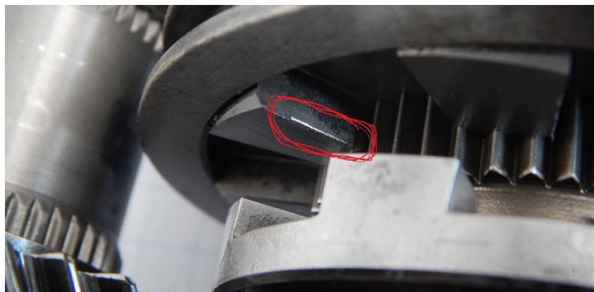
Figure 64: Rounded edge of the Maybach dog after ca. 500 gearshifts [39]
