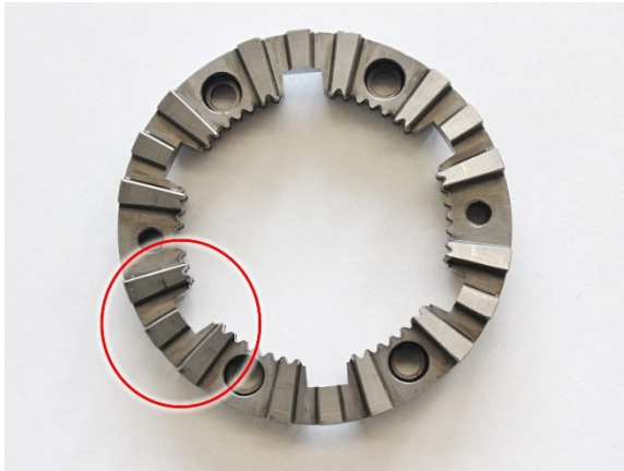
Figure 99: Sliding gear after service life test
