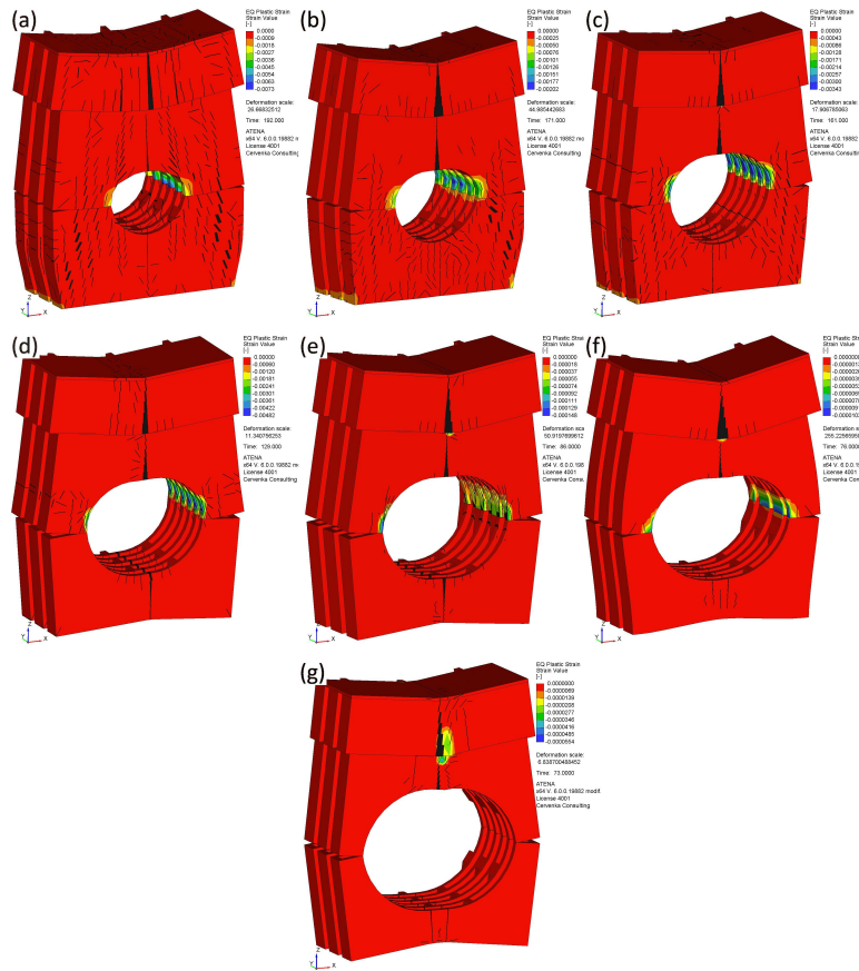
FIGURE 26. Crack pattern, deformation, and equivalent plastic strain developed in the free-standing central column with an opening diameter of (a) 250 mm, (b) 300 mm, (c) 350 mm, (d) 375 mm, (e) 400 mm, (f) 430 mm, and (g) 475 mm.
