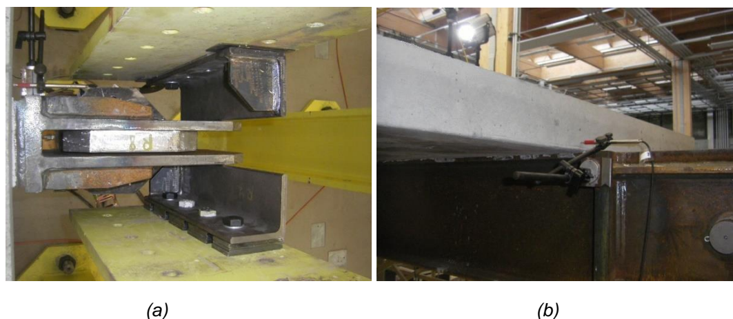
Fig. 48. Photographs of the ends of steel-concrete composite cantilevers with the displacement sensors for slip measurement - on the sagging moment side with lateral restraint of the cantilever (a), on the hogging moment side (b).
