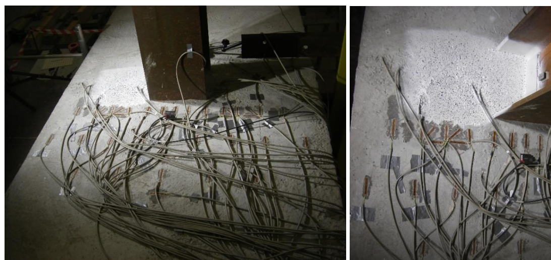
Fig. 47. Photographs of the top surface of the concrete slab with strain gauges and the surface of the slab prepared for DIC measurement.
