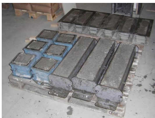
Fig. 39. SFRC test specimens.
