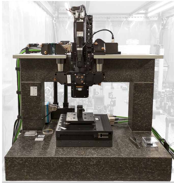
Figure 21: Commercial in-situ micromachining setup.
