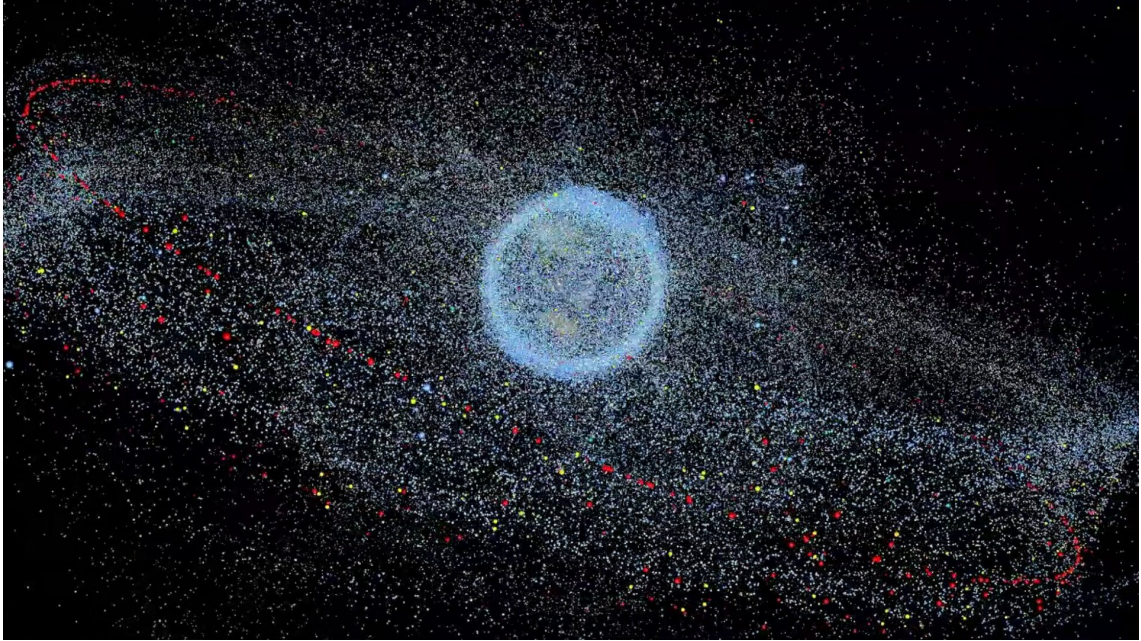
Figure 1.9: Visualisation of different types of space debris orbiting Earth with data about objects larger than 10 cm comes from the US Space Surveillance Catalogue, and for smaller objects from a statistical model made by ESA. Red dots represent satellites, yellow dots rocket bodies, green dots mission-related objects, and blue dots fragments. Different orbits, such as LEO and GEO, are visible, with LEO closely surrounding the Earth, while GEO spans furthest away. Taken from [17].
