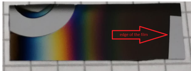
Figure 3.9: Picture of the thin film with the arrow pointing to the edge where the EDS was measured
