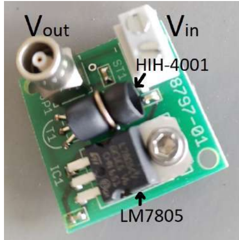
Figure 7.1: The Honeywell HIH-4001 humidity sensor connected to the LM7805 fixed-output voltage regulator IC. The regulator is supplied by voltage V_{in} and the sensor outputs voltage V_{out} .
