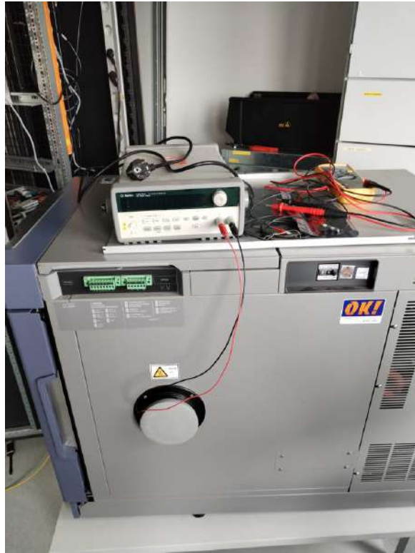
Figure 7.2: Bench-top type temperature and humidity chamber, an external voltage power supply on top together with a digital multimeter on right.
