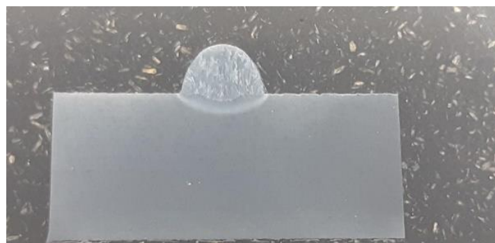
Obr. 34 – Tvar housenky – CMT – Cycle step
