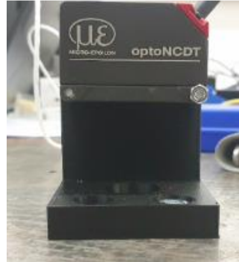
Figure 25 Laser Triangulation front view
