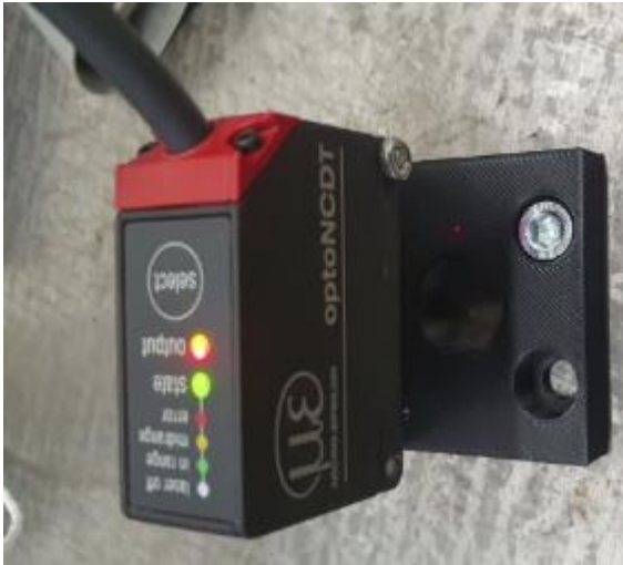
Figure 26 Laser Triangulation Glass Setup Top view
