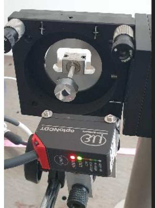
Figure 35 Laser Triangulation with Piezo Motor Setup
