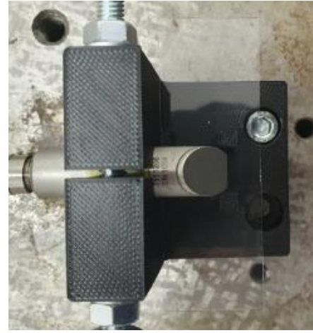
Figure 19 Confocal Glass Setup Top View
