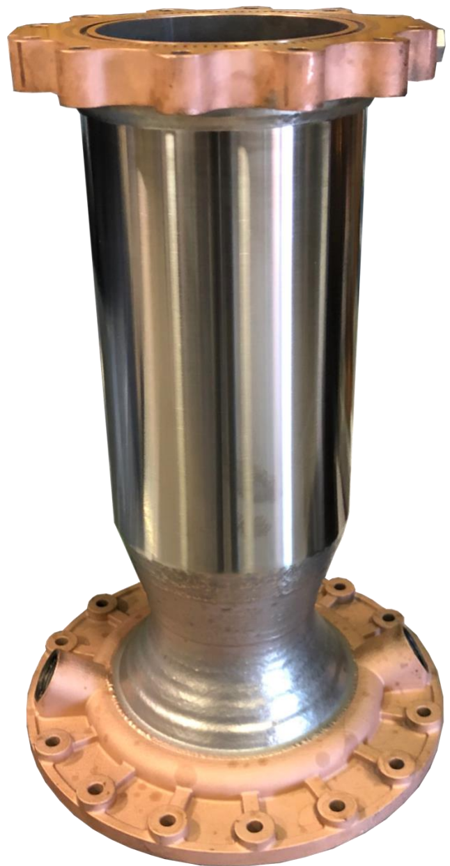
Figure 6: NASA rocket engine manufactured by CSAM [33].
