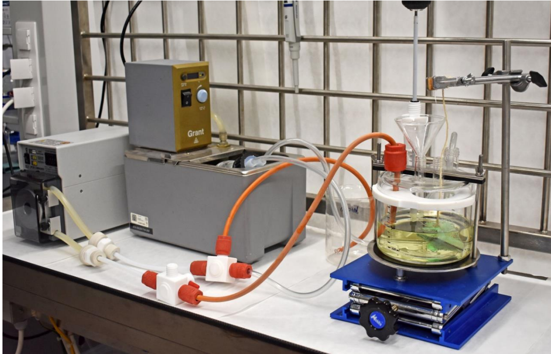
Fig. 3: Decontamination loop setup.
