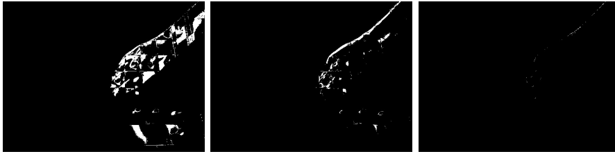
Figure 3.33: The algorithm adjusting over time to the user’s stationary hand (from left to right). It can be observed that the hand’s shadow is also detected as a movement.
