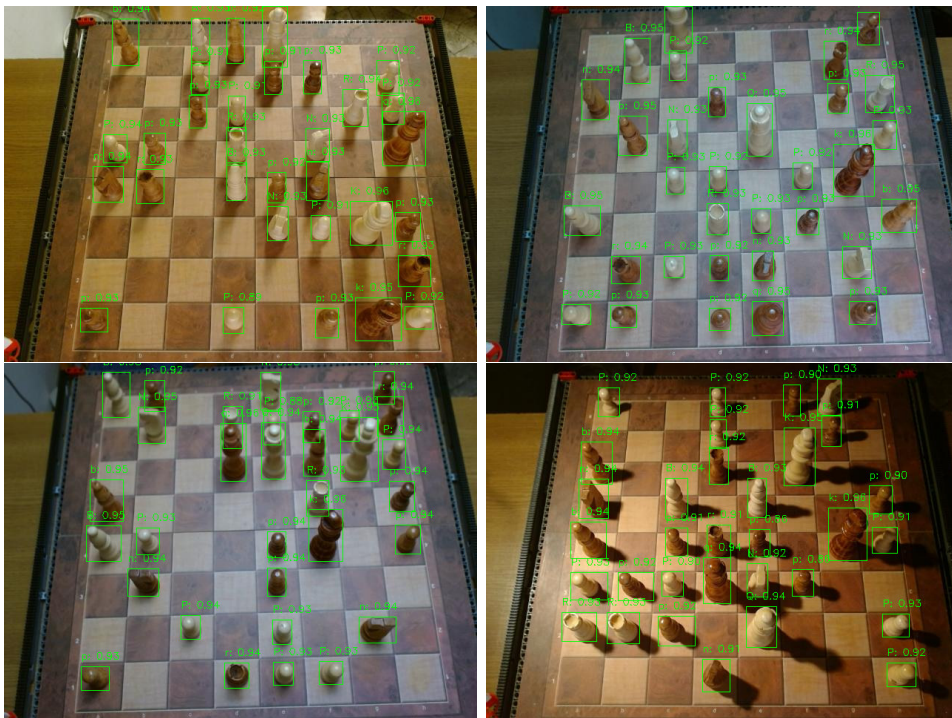
Figure 3.31: Examples of detections from the testing subset of the real-world dataset using a model trained on the YOLOv8m checkpoint. The trained model accurately detects even complex situations caused by poor lighting, misfocus, or overlapping pieces.
