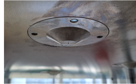
(b) : Centering cone placed on the bottom part of the shelf
