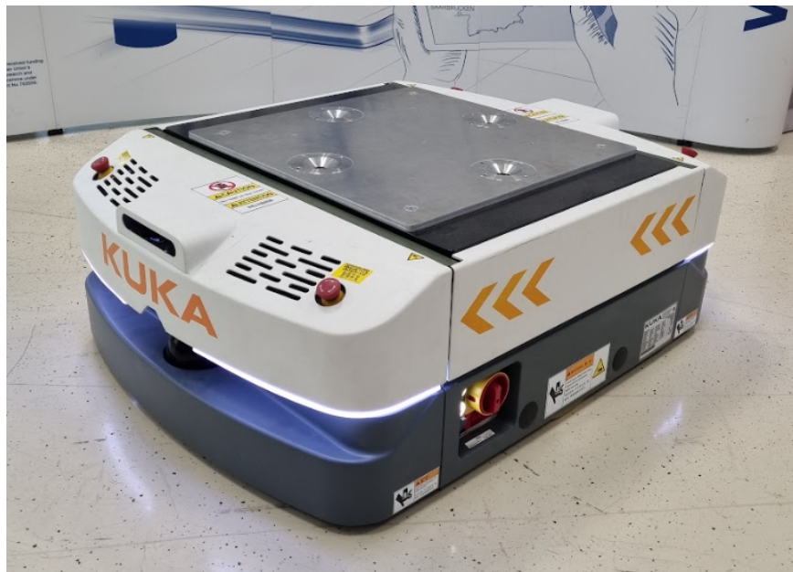
Figure 2.5: KUKA KMP600-s with additional positioning plate mounted on lift device
