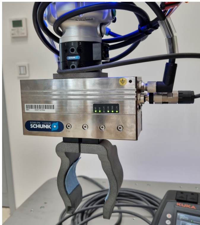
Figure 2.4: Schunk EGI 80 gripper with 3D printed fingers
