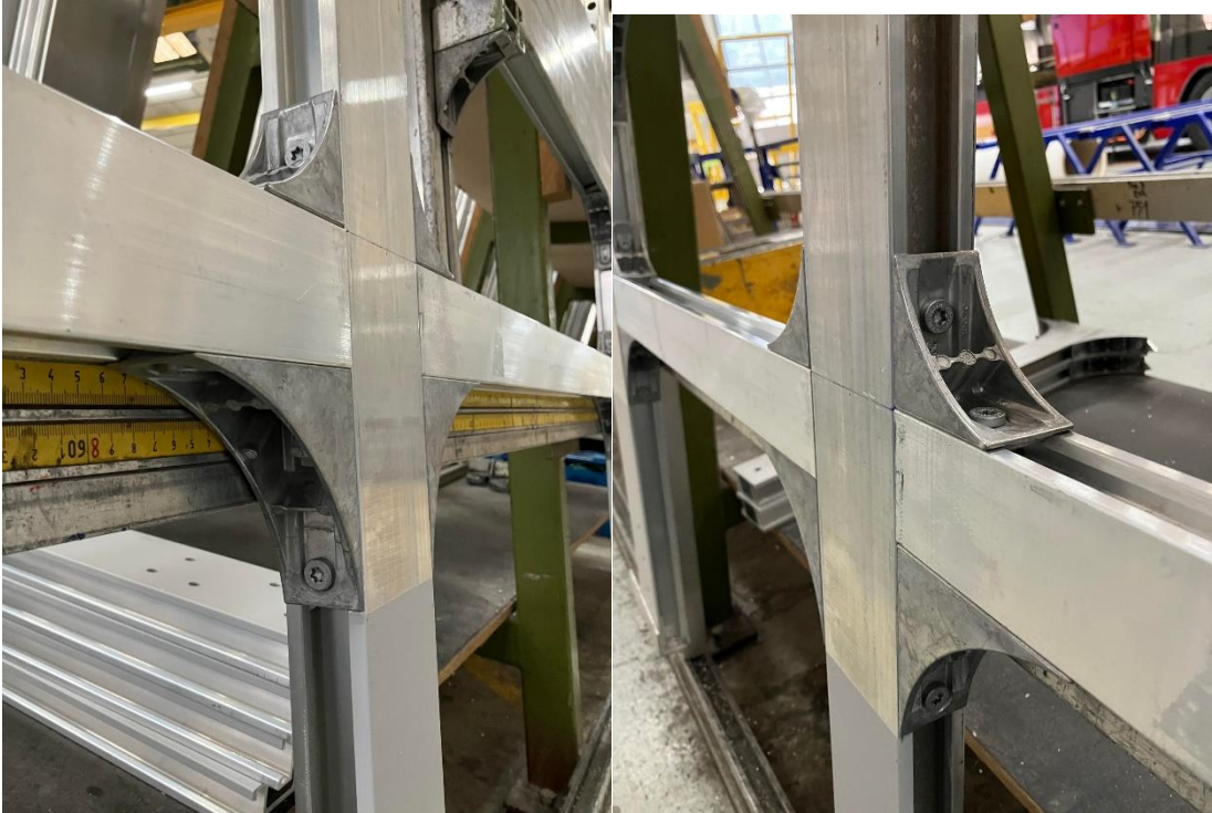
Figure 28: Picture of a connection between aluminium profiles of the body under different angles
