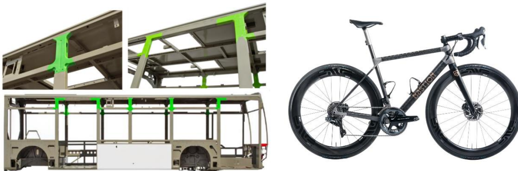
Figure 20: Two systems using the connector set solution to connect some profiles. The Mercedes bus body on the left and the Bastion Cycle bike on the right
