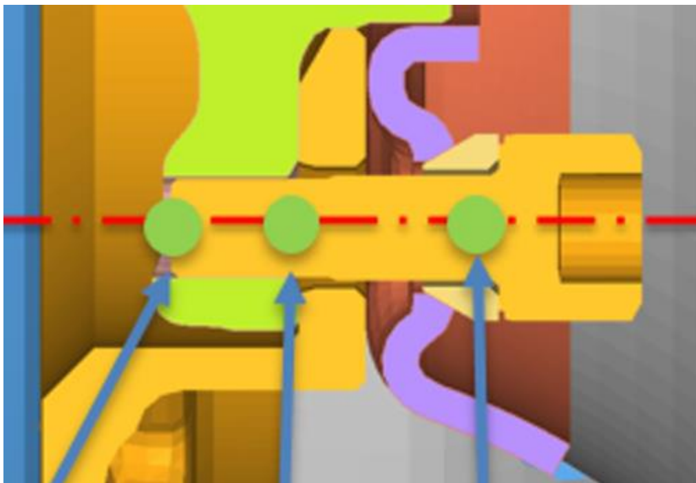
Figure 23 : Cross-section of the parts clamped by the screw
