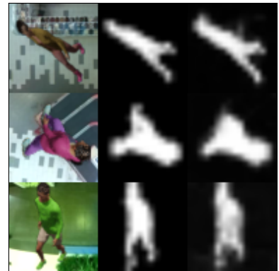
■ Figure 3.4 The first column is an input image of shape (3, 64, 64) - a synthetic person with a real background. The second column is a target segmentation mask of shape (1, 16, 16). The last column is a predicted segmentation mask of the corresponding size.
