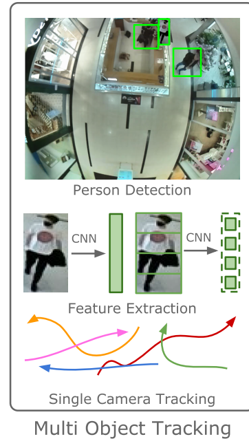
■ Figure 1.2 Single-camera multi-object tracking starts with object detection on each frame. Then runs a tracking algorithm that connects detections into sequences of the same identity. The algorithm must allow new tracks to begin and finished tracks to terminate.
